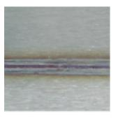
S tainless steel is recognized for its anti-corrosive properties. But the welded zones form discoloration or bluing which results in a loss of resistance to corrosion.
